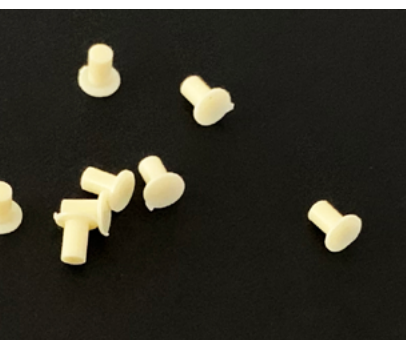
Tor's patented rivets. Once pushed through a hole, a heated press is applied and the top of the plastic rivet spreads out to trap the pieces of the movable together.
